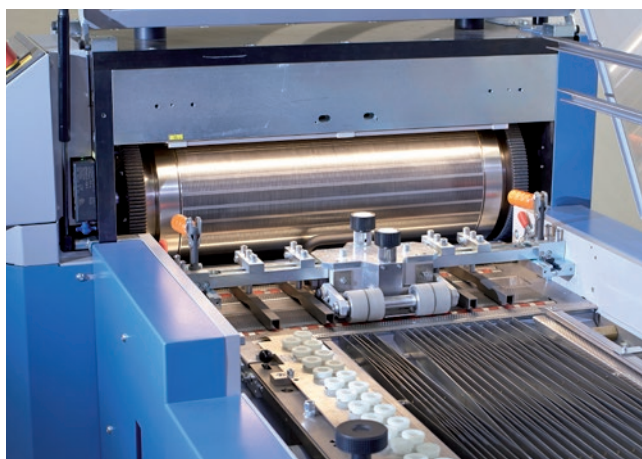
Position rollers for sheet alignment in production direction
