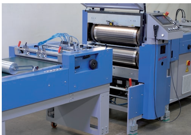
Upper and lower magnetic cylinder for the easy pick-up of flexible dies
