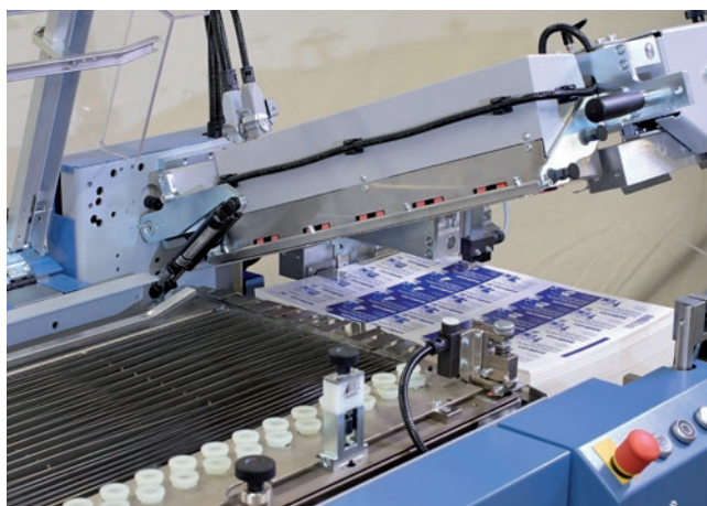
Flat pile feeder with Tornado vacuum modules
