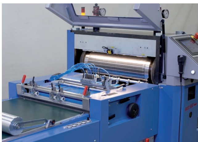
Breakout and deliver unit, adjustable without tools
