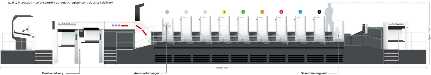
Paper can be delivered to either of two deliveries, enabling continuous press operation while delivering printed sheets. Can also be used to separate paper waste.
