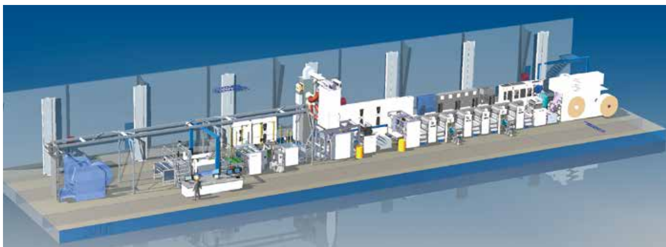
KCM production line, from the unwinder to the stacker delivery in the typical right to left layout. KCM is the master of all printing processes and can combine them, like here with a flexo unit after the offset units for varnish management.
